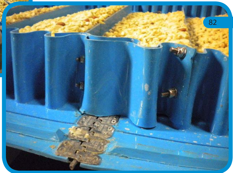
SD with Sidewalls, Flights and Metal Lace in Peanuts processing
