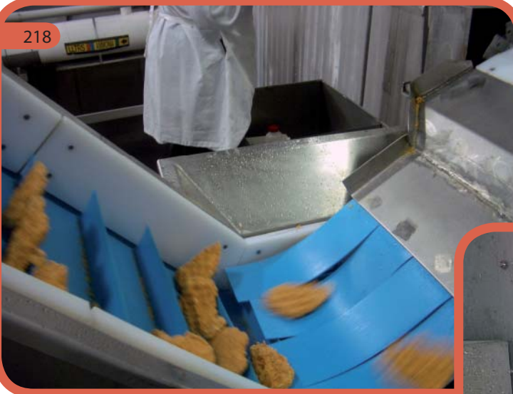
FMB/W, FHB/W, FL/W Volta belts used as Skirts/Scrapers on Conveyor
