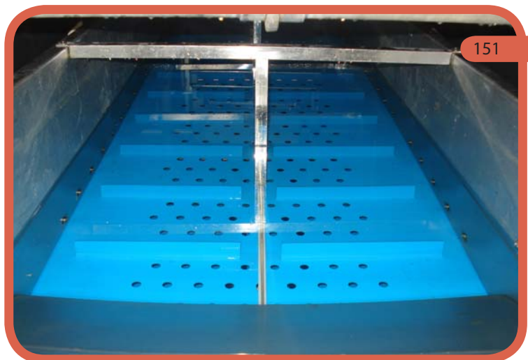
Perforated FMB belt working under water
