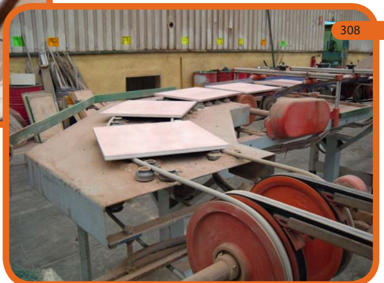
RPZS/PRS profile for Floor tile Conveying
